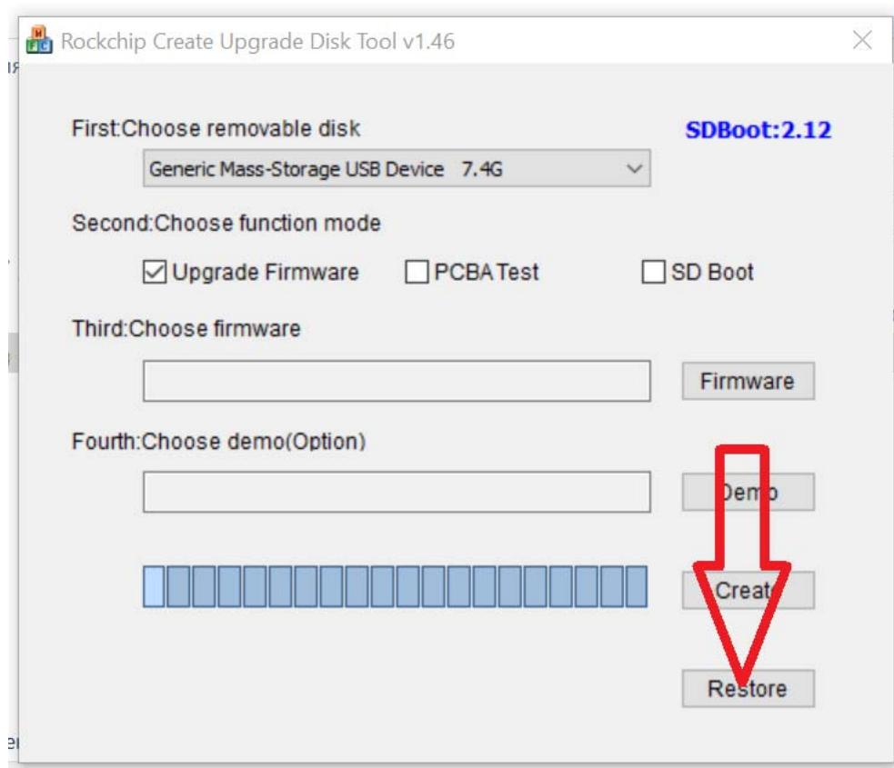
Create a second USB flash drive. A flash drive must necessarily be formatted in **FAT32 !!!**
