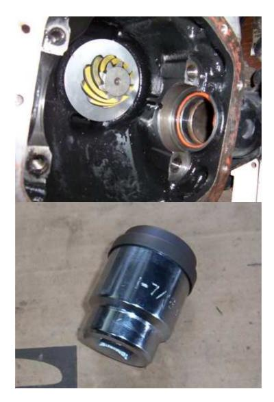
This photo shows the seal removed. The orange ring is not part of the seal so leave in place. To install the new seal I used a 1-7/16" socket, by the look of the photo, that fitted inside the seal nicely.
