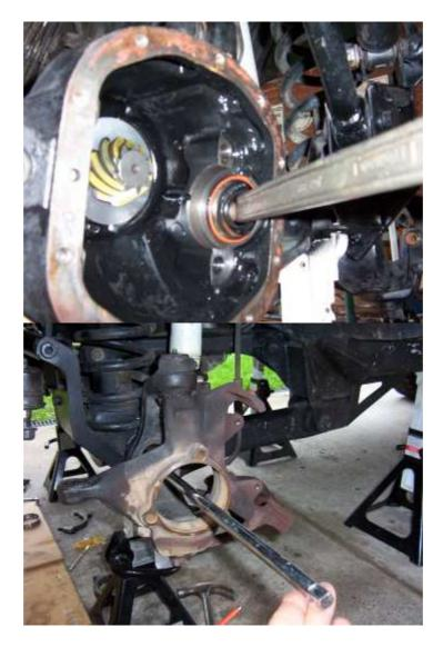
You can pry the seal out from the front side or tap it out using a socket extension instead. I found the second way a bit easier.
